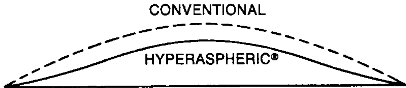
Conventional Lens vs. Full Field Aspheric Fig 3-8
