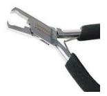
2) Trim compression sleeve (FROM BACK OF LENS). BE VERY CAREFUL NOT TO SCRATCH LENS. When cutting the plastic compression sleeve,
