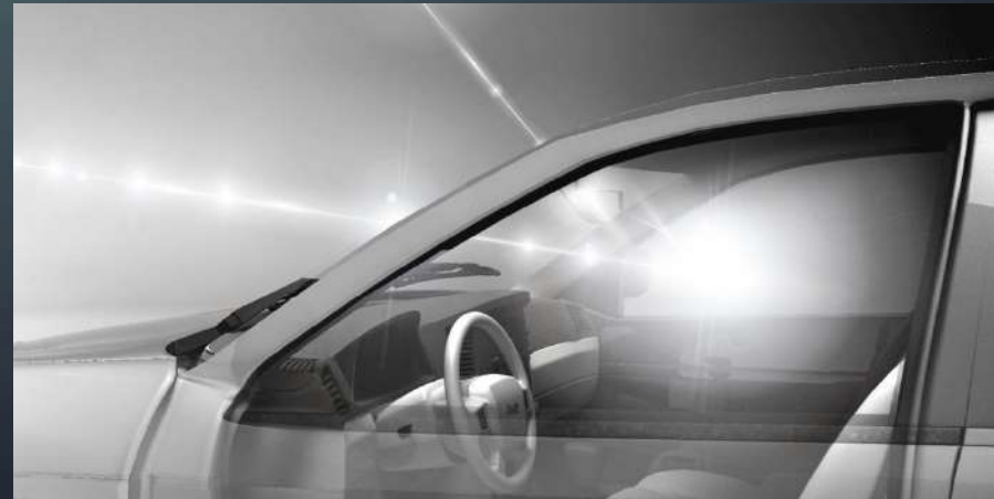
Reflection from mirror hardware and glare light directly from the sun/sky
